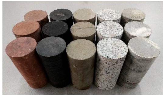
Figure 2. Prepared rock samples for uniaxial cyclic compression tests.
