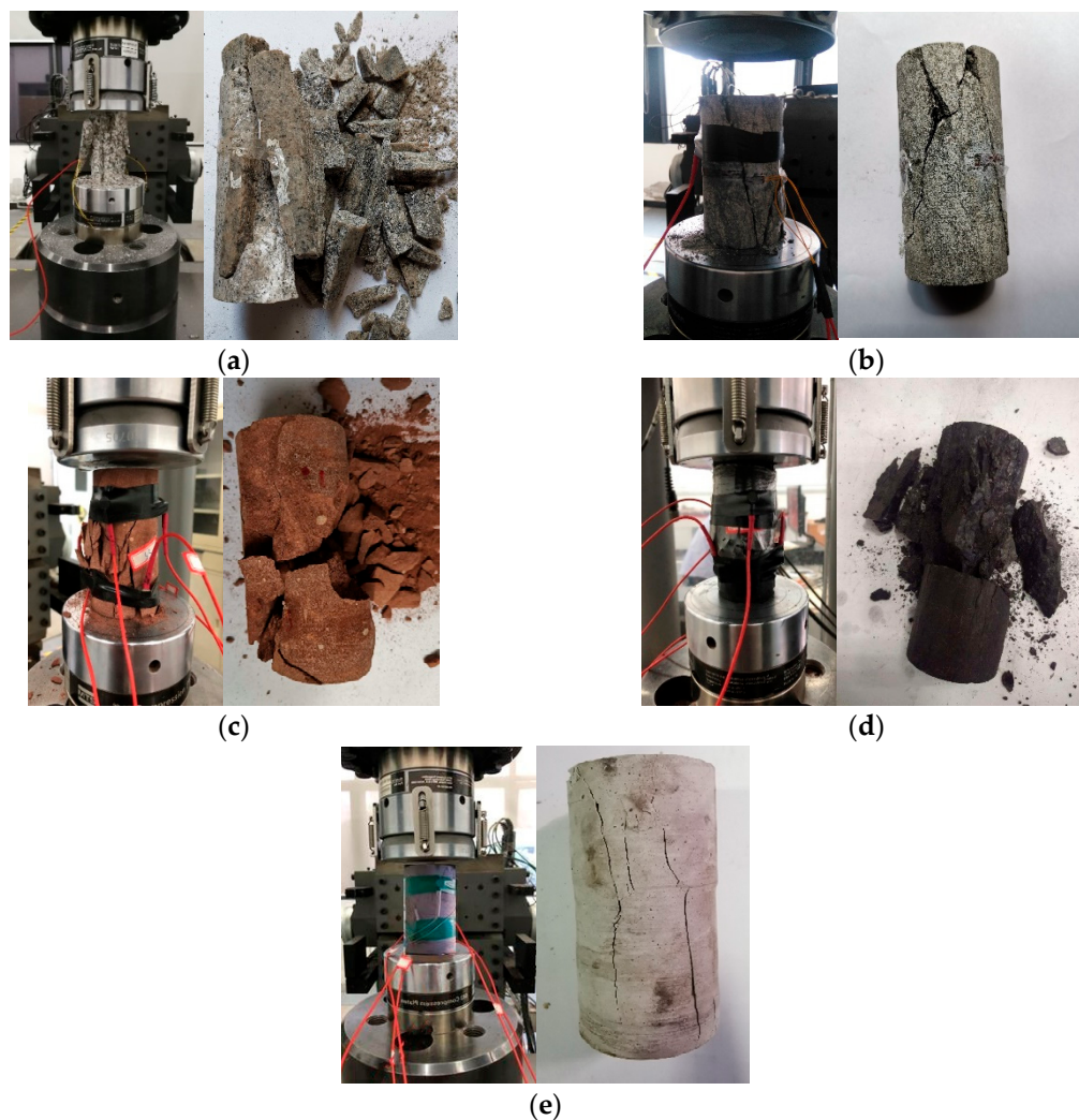
Figure 14. Failure mode of five rock materials. (a) Granite, (b) gypsum, (c) red sandstone, (d) coal, and (e) high-water material.
