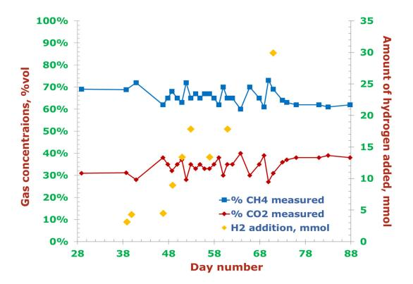
**Figure 2.** Effect of  $H_2$  injection on biogas composition (v/v) in terms of standard temperature and pressure (STP) normalized CH<sub>4</sub> and CO<sub>2</sub> contents.
