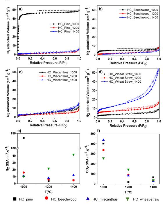
**Figure 6.** N<sub>2</sub> adsorption/desorption isotherms for (**a**) pine, (**b**) beechwood, (**c**) miscanthus and (**d**) wheat straw derived hard carbons. (**e**) N<sub>2</sub> and (**f**) CO<sub>2</sub> specific surface area (SSA) variation with temperature for all the hard carbons.
