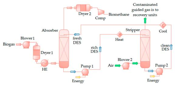
Figure 2. Scheme for the biogas upgrading technology [55,56].
