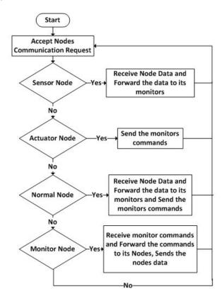
Figure 22. Server (broker) flowchart.
