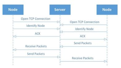
Figure 10. Sequence diagram for node to node communication.
