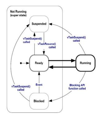
Figure 17. Task state diagram.
