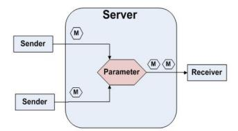
Figure 27. Data decoupling.
