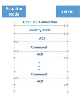
Figure 7. Sequence diagram for an actuator node.
