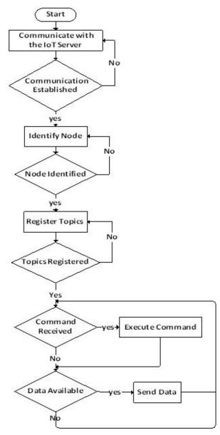
Figure 21. Normal node flowchart.
