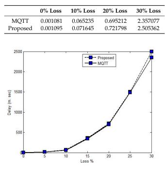
Figure 23. The average message delay (in seconds).
