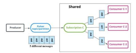
Figure 3. Multi-messages technique using batching; for example, pulsar.apache.
