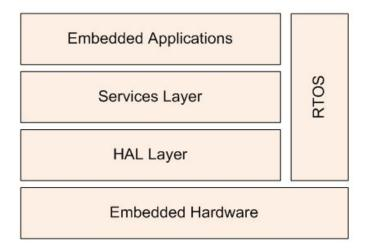
Figure 15. Real-time operating system (RTOS) architecture.
