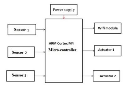
Figure 18. Block diagram of the proposed embedded IoT client.
