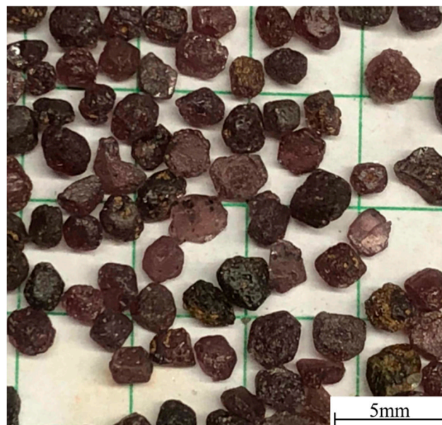
Figure 4. Magnified view of garnets on 5 mm square grid. The garnet size and roundness evolved during experiments so that fresh garnet had to be replaced in the system regularly. The observed rate of material removal was linear over the 110 h of testing [30].
