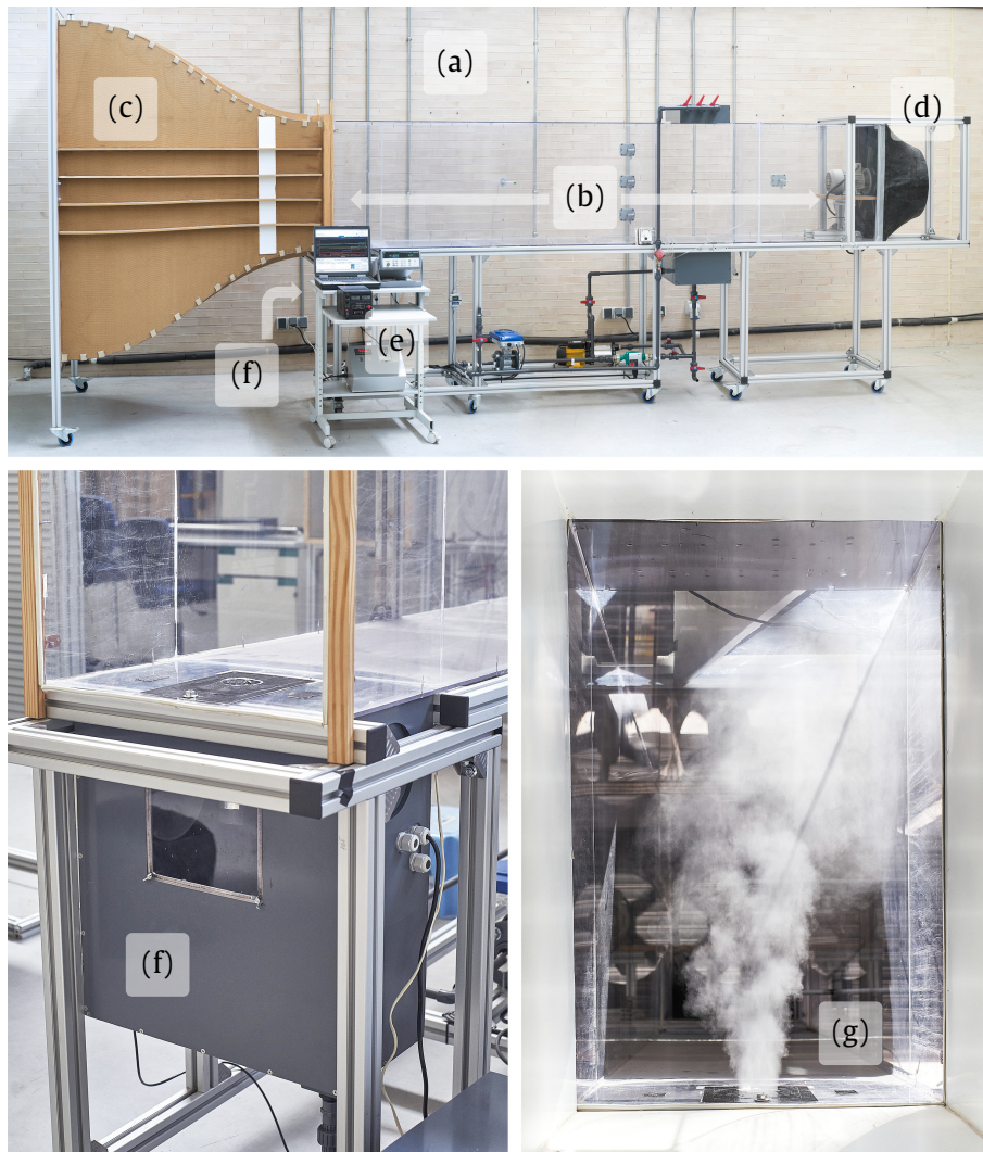
Figure 2. Subsonic wind tunnel facility employed in the experimental tests: (a) subsonic wind tunnel; (b) test section; (c) nozzle; (d) diffuser; (e) data acquisition system; (f) ultrasonic mist generator; and (g) structure of water mist stream.
