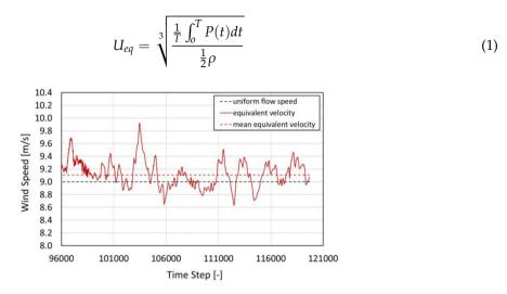
**Figure 2.** Comparison between a uniform wind speed, a real fluctuating one and its equivalent speed as in Equation (1).
