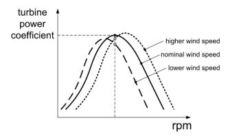
**Figure 3.** Schematic representation of the variation of turbine power coefficient due to a local variation of the incoming wind velocity at a fixed revolution speed.
