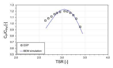
**Figure 13.** Comparison between the experimental turbine power curve (in dimensionless form) in turbulence and the predictions using the VARDAR code: the BEM code is run with the airfoil polars obtained for a 9.5% turbulence condition and at the equivalent wind speed of 9.2 m/s.
