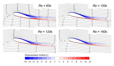
**Figure 12.** Vorticity contours and velocity streamlines around the blade at 15° incidence for different Reynolds.
