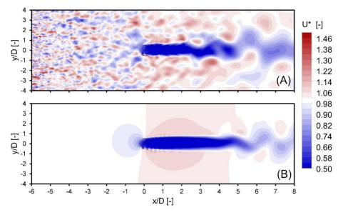
**Figure 1.** Computed contours for the dimensionless streamwise velocity: (**A**) turbine simulation with turbulence, and (**B**) turbine simulation without turbulence.
