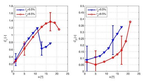
Figure 7. Experimental polars for the virtually cambered airfoil at *Re* = 80 k.
