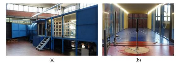
**Figure 4.** (a) Wind tunnel with a wooden grid for turbulence generation installed; (b) analyzed wind turbine.
