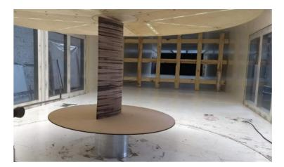
**Figure 5.** Airfoil model mounted inside the FLOW wind tunnel, with the turbulence grid installed in the background.
