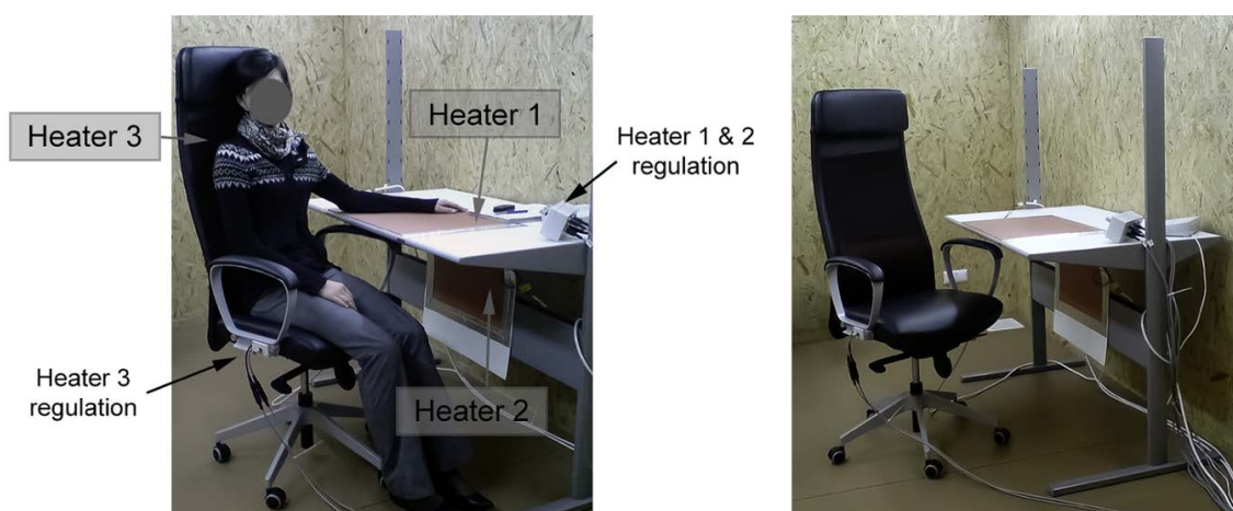
Figure 1. Workstation incorporating three heating mats (heaters).
