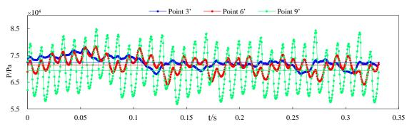
Figure 26. Pressure fluctuation in the vortex.
