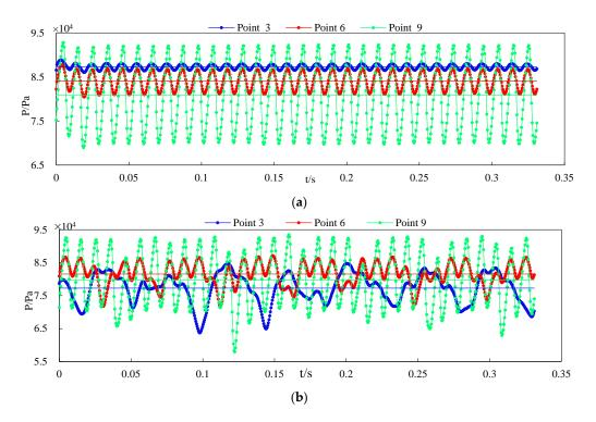
Figure 24. Time-domain diagram of the impeller inlet monitoring points: (a) Without VGs; (b) With VGs.
