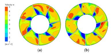
Figure 18. Axial velocity distribution diagram inside the guide vane: (a) Without VGs; (b) With VGs.
