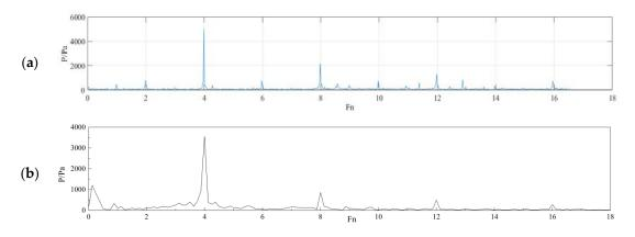
**Figure 11.** Frequency-domain diagram of the pressure fluctuations: (**a**) Experiment; (**b**) Numerical simulation. Fn in the figure is a multiple of the impeller rotation frequency.
