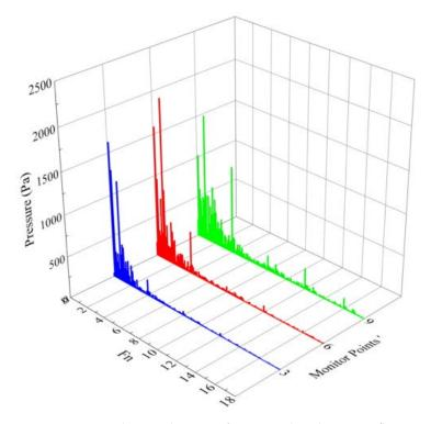
Figure 28. Frequency domain diagram of vortex-induced pressure fluctuation.
