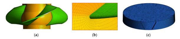
Figure 5. Figures of grids: (a) Impeller; (b) Grid refinement of impeller tip; (c) VGs.
