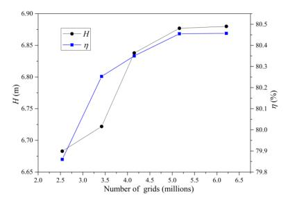
Figure 4. Analysis of grid independence for the pump device.
