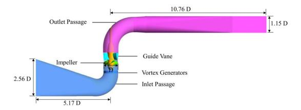
Figure 2. Layout of the vertical pump device.
