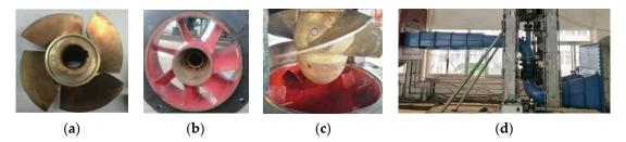
Figure 8. Picture of experiment: (a) Impeller; (b) Guide vane; (c) VGs; (d) Pump device.
