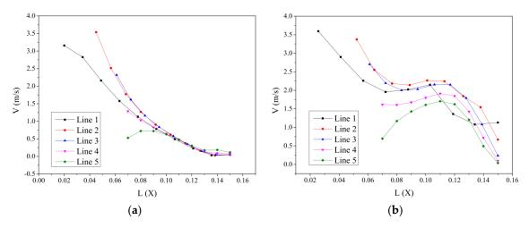
Figure 13. Radial velocity of the impeller inlet: (a) Without VGs; (b) With VGs.
