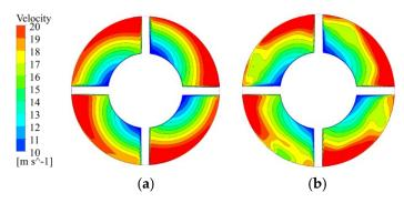
Figure 17. Velocity distribution diagram inside the impeller: (a) Without VGs; (b) With VGs.
