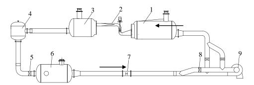
**Figure 7.** Layout of the experimental test system. 1. inlet tank 2. test segment schematic diagram 3. outlet tank 4. bifurcation tank 5. working condition adjustment gate valve 6. regulating rectifier 7. electromagnetic flowmeter 8. system that runs the control gate valve in forward and reverse directions 9. auxiliary pump unit.
