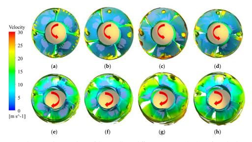
**Figure 21.** The internal vortex shape of the impeller at different moments: (**a**–**d**) See from the direction of the impeller inlet that the blades rotate counterclockwise; they are rotated by  $0^{\circ}$ ,  $30^{\circ}$ ,  $60^{\circ}$  and  $90^{\circ}$ , respectively; (**e**–**h**) See from the direction of the impeller outlet that the blades rotate clockwise; they are also rotated by  $0^{\circ}$ ,  $30^{\circ}$ ,  $60^{\circ}$  and  $90^{\circ}$ , respectively.
