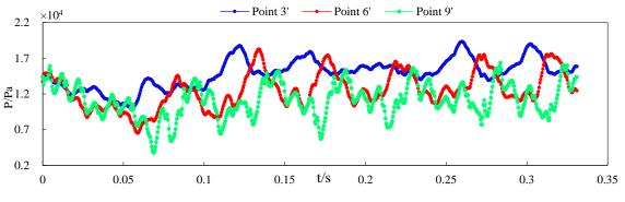
Figure 27. Time-domain diagram of vortex-induced pressure fluctuation.
