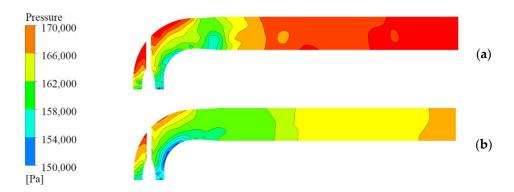
Figure 19. Outlet passage pressure distribution: (a) Without VGs; (b) With VGs.
