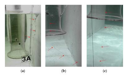
Figure 1. Pictures of vortices: (a) Surface vortex; (b) Wall-attached vortex; (c) Bottom-attached vortex.
