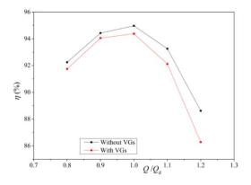
Figure 16. Comparison diagram of the impeller efficiency with and without VGs.
