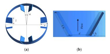
Figure 3. Dimensional drawings of fixed VGs: (a) Top view; (b) Right view.
