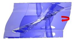
Figure 22. Shape of the vortex in the impeller.
