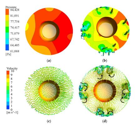
**Figure 20.** Inlet flow field of the impeller: (a) Pressure contour diagram without VGs; (b) Pressure contour diagram with VGs; (c) Velocity vector and vortex diagram without VGs; (d) Velocity vector and vortex diagram with VGs.
