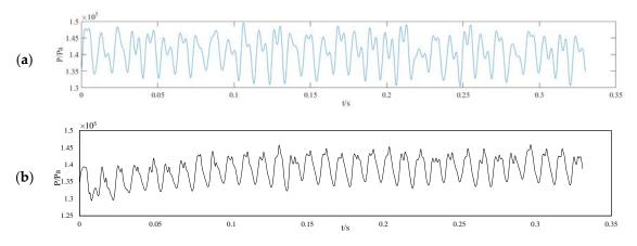
Figure 10. Time-domain diagram of pressure fluctuation: (a) Experiment; (b) Numerical simulation.
