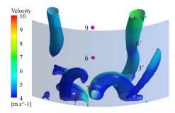
Figure 25. Positions of the vortex and monitoring points.
