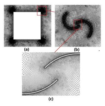
**Figure 4.** Relative rotation positions around the blades at different rotor angles. (**a**) Domain mesh; (**b**) rotor mesh; (**c**) boundary layer mesh.
