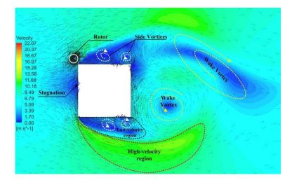
**Figure 6.** Contours and vectors of velocity around the building for the case of l = 1.5 D,  $\phi = 45$  and TSR = 1.
