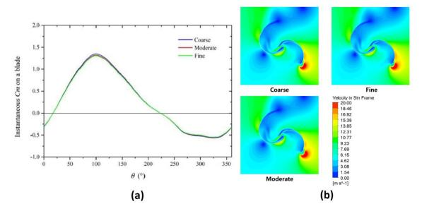
**Figure 7.** Mesh density verification. (**a**) Cm of a blade under different grid numbers; (**b**) velocity distribution under different grid numbers.
