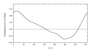
**Figure 18.** The instantaneous coefficient of torque on a blade at  $\phi = 0^{\circ}$  and TSR = 0.4.
