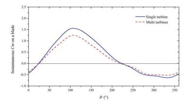
**Figure 15.** Effects of adjacent turbines on the instantaneous torque on a blade at TSR = 1.0, l = 1.00 D and  $\phi = 45^{\circ}$ .
