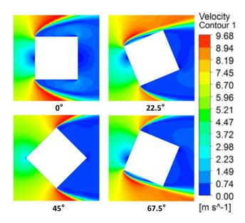
Figure 9. Contours of velocity around the building under different wind directions.
