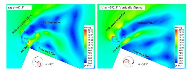
**Figure 22.** Velocity contours around the turbine at TSR = 1.2 and at (**a**)  $\theta = 90^\circ$ ,  $\phi = 67.5^\circ$  and (**b**)  $\theta = 345^\circ$ ,  $\phi = 292.5^\circ$ .
