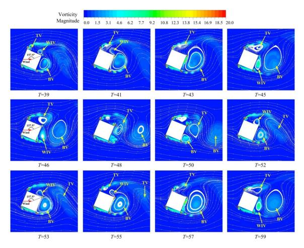
**Figure 24.** Contours of vorticity and streamlines around the building at  $\phi = 157.5^{\circ}$ .
