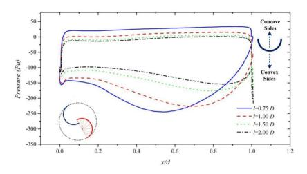
**Figure 13.** Pressure distribution on the blade at  $\theta$  = 120° and at different installation positions.
