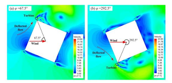
**Figure 20.** Velocity contours around the building at TSR = 1.2 and at (**a**)  $\phi = 67.5^{\circ}$  and (**b**)  $\phi = 292.5^{\circ}$ .
