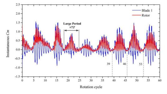
**Figure 23.** Instantaneous coefficients of torque on both the blade and the turbine at TSR = 0.4 and  $\phi = 157.5^{\circ}$ .
