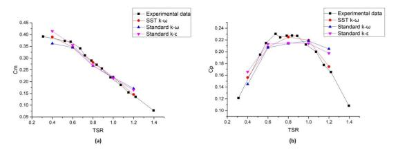
**Figure 8.** Numerical method validation. (**a**) Validation of the turbine torque; (**b**) validation of the turbine power.
