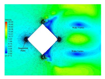
**Figure 19.** Velocity contours and vectors around the building at  $\phi = 0^{\circ}$  and TSR = 0.4.
