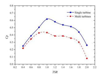
Figure 14. Effects of adjacent turbines on the power performance of the turbine.
