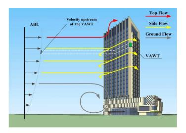
Figure 1. A schematic of a VAWT mounted on the edge of a building.
