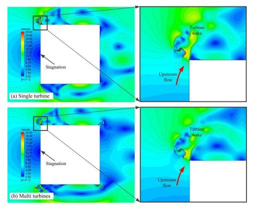
**Figure 16.** Contours of velocity at l = 0.75 D, TSR = 1.0,  $\phi = 45^{\circ}$  and  $\theta = 120^{\circ}$ .
