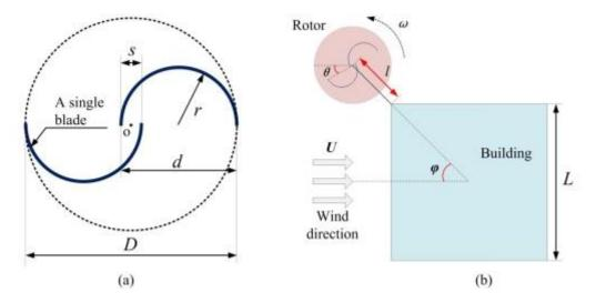
**Figure 2.** Parameters of the Savonius turbine (the rotor and the building are not scaled). (**a**) Structural parameters of the Savonius rotor; (**b**) operational parameters of the Savonis rotor.
