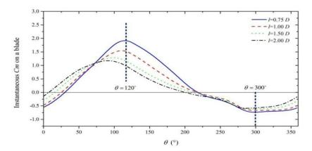
Figure 11. Instantaneous coefficients of torque on a single blade at different gaps.
