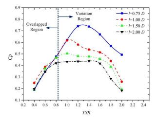
Figure 10. The power performance of turbines at different gaps.
