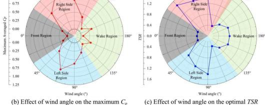
**Figure 17.** Plots of the maximum  $C_p$  and the optimal *TSR* with respect to the wind angle.
