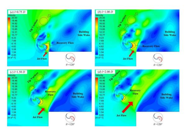
**Figure 12.** Contours of velocity near the turbines at  $\theta = 120^{\circ}$  and at different installation positions.
