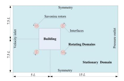
Figure 3. Computational domains and boundary conditions (the display is not scaled).
