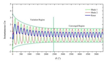
**Figure 5.** The torque coefficients during 15 rotation periods for the case of l = 1.5 D,  $\phi = 45$  and TSR = 1.
