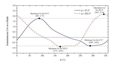
**Figure 21.** Instantaneous coefficients of torque on a blade at  $\phi = 67.5^{\circ}$  and  $292.5^{\circ}$  for TSR = 1.2.
