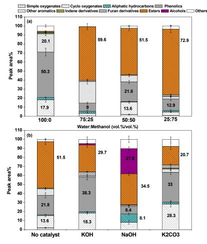
**Figure 7.** Selectivity to various functional groups in bio-crude obtained at (**a**) different water-to-methanol ratios and (**b**) different alkali catalysts at water:methanol of 50:50 (vol.%/vol.%). The final temperature is 300 °C, reaction time is 60 min, and rice-straw-to-solvent ratio is 1:10 wt./wt.
