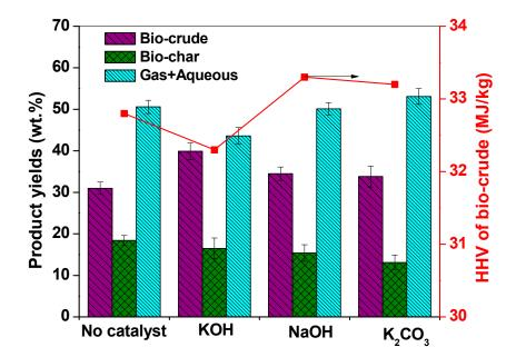
**Figure 4.** Effect of alkali catalysts on product yields and HHV of bio-crude at 300 °C, 60 min, rice straw:solvent ratio of 1:10 wt./wt., catalyst quantity of 5 wt.%, and 50:50 (vol.%/vol.%) methanol:water.
