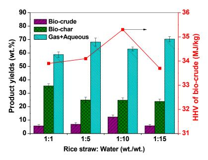
**Figure 2.** Effect of rice-straw-to-water ratio on product yields and HHV of bio-crude at a final temperature of 300 °C and 60 min.
