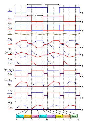
Figure 3. Theoretical waveforms of the proposed converter.
