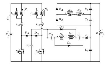
Figure 2. Equivalent circuit of the proposed converter.
