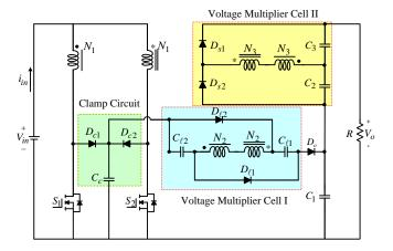
Figure 1. Circuit configuration of the proposed converter.
