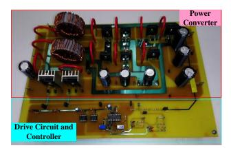
Figure 20. Photograph of the laboratory prototype.
