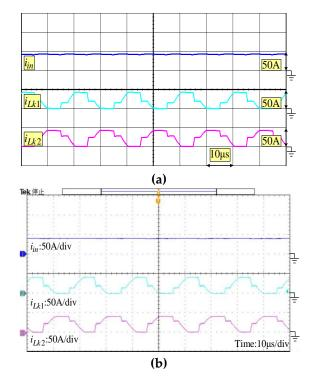
**Figure 14.** Waveforms of  $i_{in}$ ,  $i_{Lk1}$  and  $i_{Lk2}$ . (a) Simulated results. (b) Experimental results.
