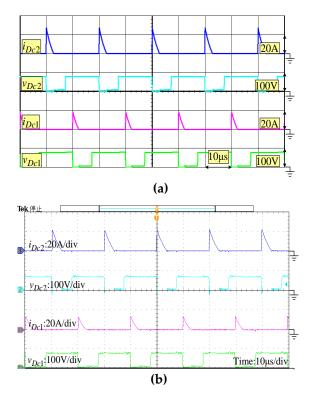
**Figure 15.** Waveforms of  $i_{Dc1}$ ,  $v_{Dc1}$ ,  $i_{Dc2}$  and  $v_{Dc2}$ . (a) Simulated results. (b) Experimental results.
