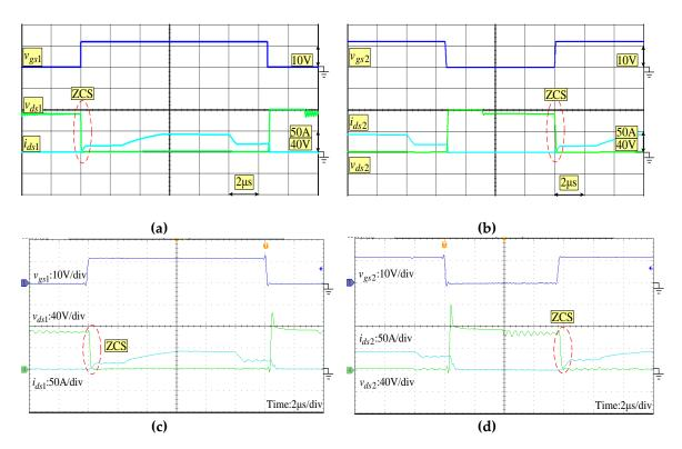
**Figure 16.** Waveforms of the ZCS turn-on for switches  $S_1$  and  $S_2$ . (**a**) and (**b**) simulated results. (**c**) and (**d**) experimental results.
