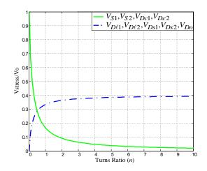
Figure 6. Normalized voltage stresses on semiconductor devices.
