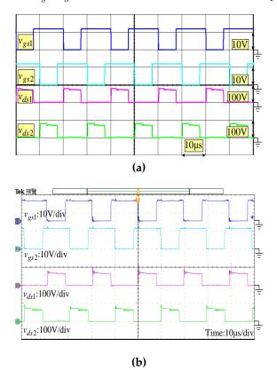
**Figure 13.** Waveforms of  $v_{gs1}$ ,  $v_{gs2}$ ,  $v_{ds1}$  and  $v_{ds2}$ . (a) Simulated results. (b) Experimental results.
