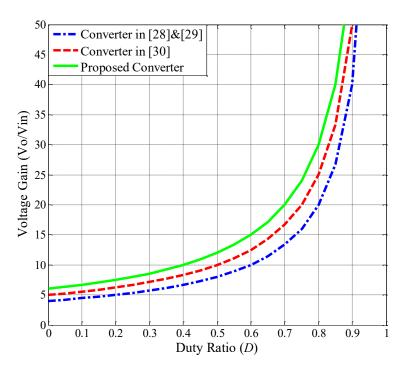
**Figure 7.** Voltage gain comparison with turns ratio n = 1.
