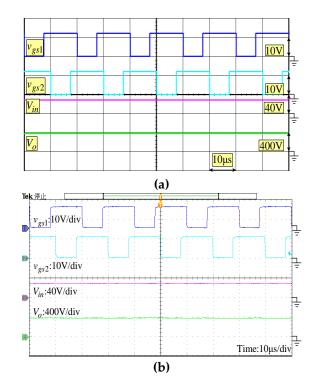
**Figure 12.** Waveforms of  $v_{gs1}$ ,  $v_{gs2}$ ,  $V_{in}$  and  $V_o$ . (a) Simulated results. (b) Experimental results.
