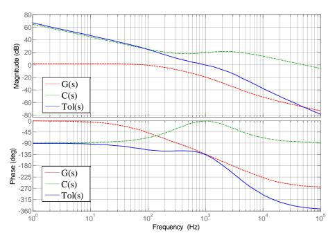
Figure 11. Bode plots of plant, controller and loop gain.
