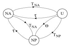
**Figure 1.** Graph of a model of an object's operation process with a servicing system which uses an artificial neural network which processes diagnostic information expressed in a trivalent evaluation of states.
