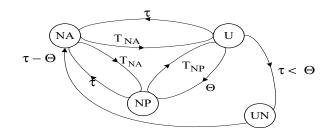
**Figure 3.** Graph of a model of an operation process of wind power plant with a maintenance system that is classically organized without any examination of the state in the assessment process.
