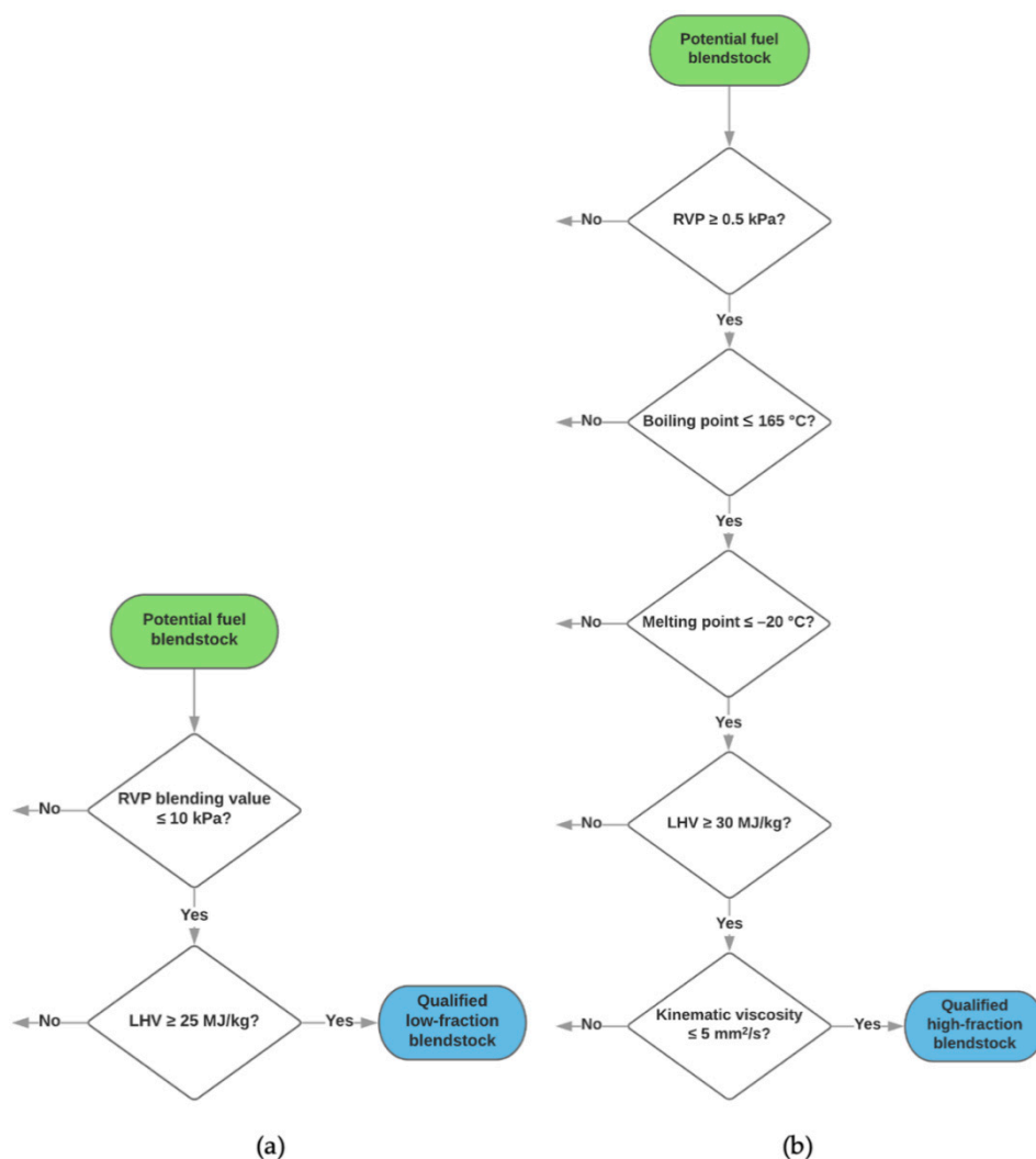
Figure 2. Decision framework for the second-stage screening of the alcohol database. (a) Low-range blends (Scenario 1). (b) High-range blends (Scenario 2).
