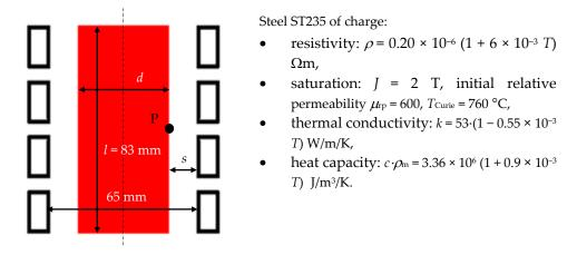
**Figure 5.** Example of an IHS with a four-turn inductor.
