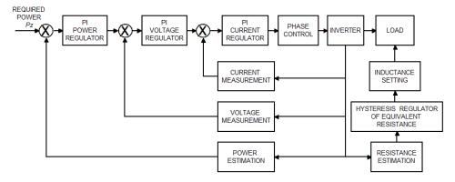
Figure 13. Block diagram of the cascade power regulator in the induction heating generator model.
