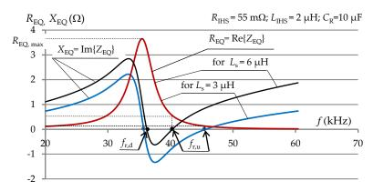
**Figure 2.** The waveforms of the equivalent resistance and reactance of the LLC system as a function of frequency.
