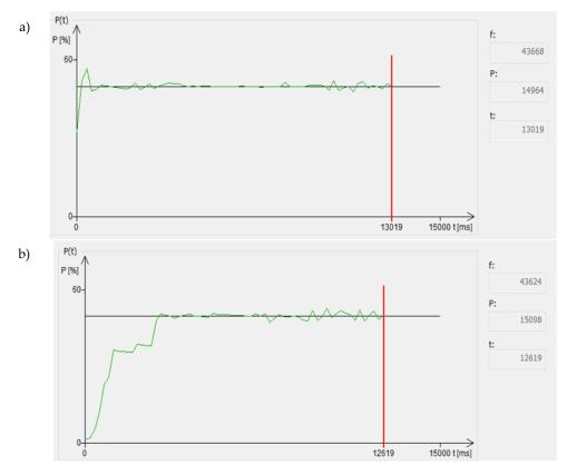
**Figure 15.** Visualization of the generator power waveform during the heating process: (a) with the initial load identification procedure and (b) with a starting frequency that differs by 5% from that established in the load identification procedure.
