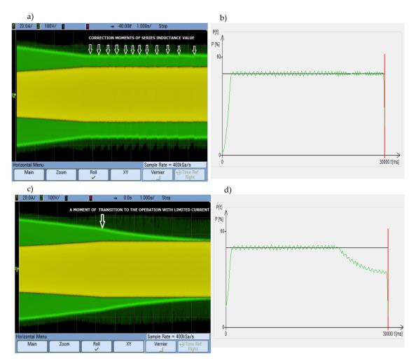
**Figure 16.** Current, output voltage and power waveforms for one module of the generator inverter during the heating process: ( $\mathbf{a}$ , $\mathbf{b}$ ) with  $L_{\rm s}$  the change procedure enabled and ( $\mathbf{c}$ , $\mathbf{d}$ ) without changing the  $L_{\rm s}$  settings.
