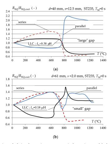
**Figure 7.** Comparison of relative changes in resonance equivalent resistance of the load as a function of the charge surface temperature during heating by an inverter with different types of resonance system: (a) "large" gap and (b) "small" inductor–charge gap.
