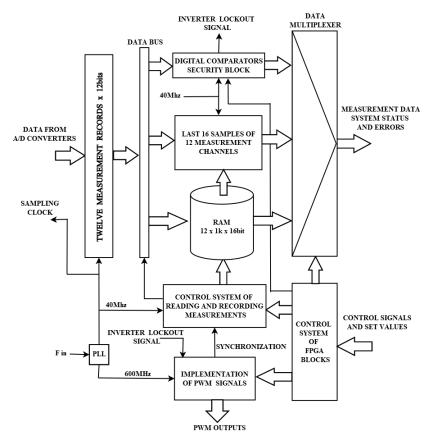
Figure 12. Block diagram of the FPGA structure.
