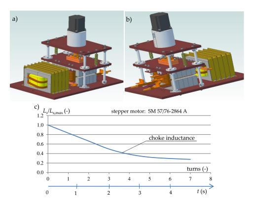
**Figure 9.** Structural model of the magnetic assembly with a stepper motor: (a) view from the transformer side, (b) view from the choke side, and (c) choke inductance change as a function of stepper motor turns.
