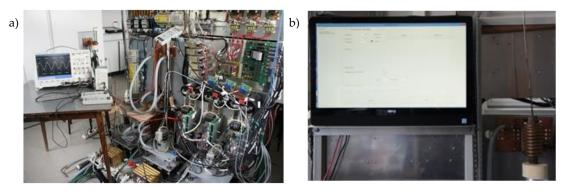
**Figure 14.** Photograph of the model of the generator for induction heating with a controlled LLC system: (a) back side and (b) front side.
