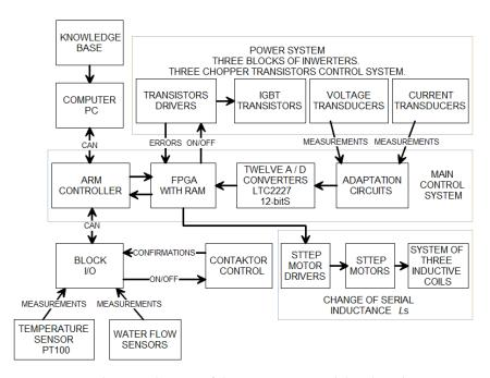
**Figure 11.** Schematic diagram of the generator control distributed structure.
