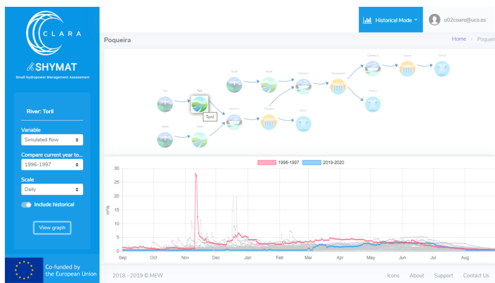
Figure 5. Example of visualization of the SHYMAT web-user interface. Historical mode outputs: The river element is selected in the topology panel and a graph showing the daily streamflow data for the hydrological years 1996/97 (red) and 2019/20 (blue), and for the period 1981–2020 (grey) appears on the screen.
