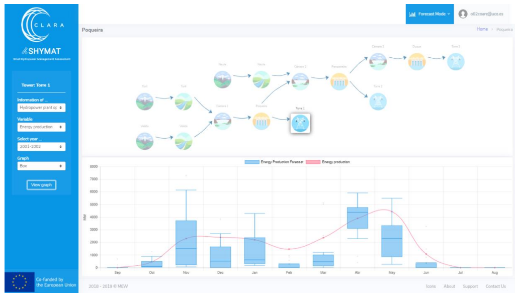
Figure 8. Example of the visualization of the SHYMAT web user interface. Forecast mode outputs: The power gridelement is selected in the topology panel and a graph showing monthly values of the energy production expected for the next seven months (boxplot) and real energy production (line) appears on the screen.
