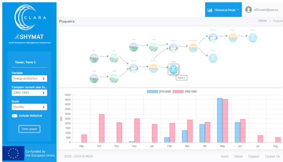
Figure 6. Example of the visualization of the SHYMAT web-user interface. Historical mode outputs: The power grid element is selected in the topology panel and a graph showing the monthly energy production data for the hydrological years 1992/93 (red) and 2019/20 (blue) appears on the screen.
