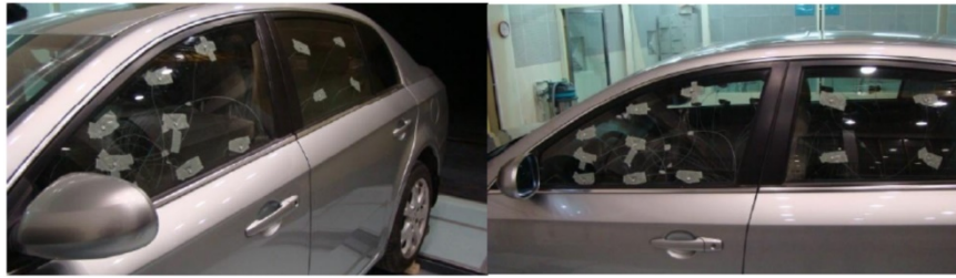
Figure 3. Layout to measure surface pressure.
