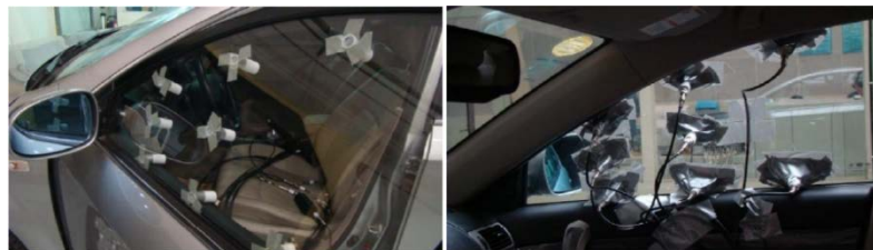
Figure 7. Layout to measure noise intensity.
