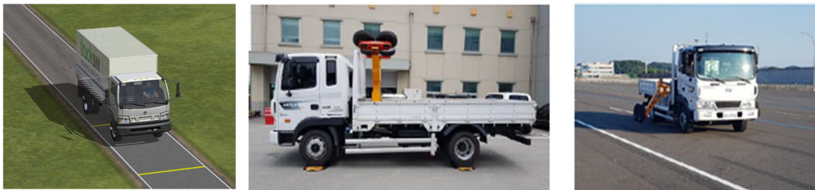
Figure 4. TruckSim model and actual vehicle for H-Mega Truck.
