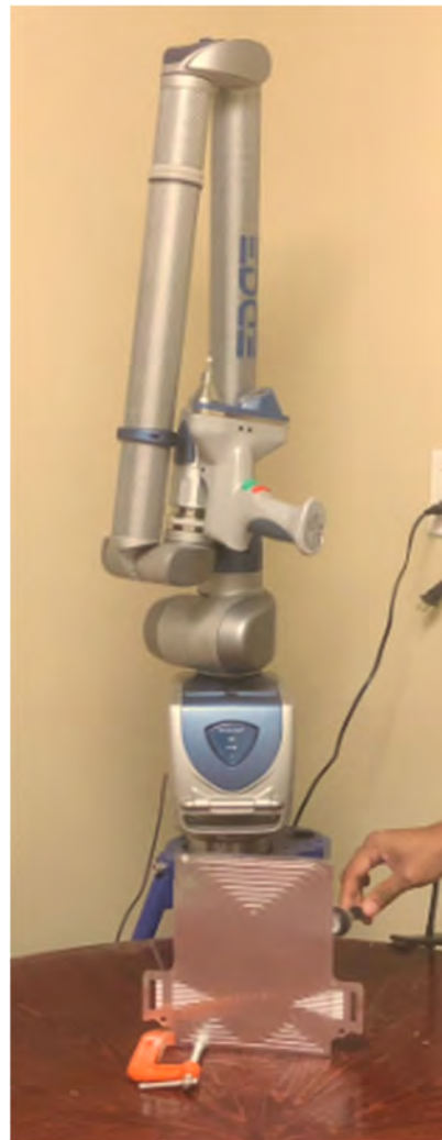
Figure 2. Laser scanning set-up.
