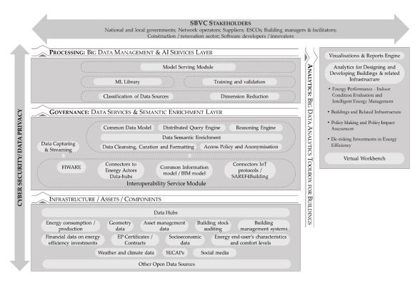
Figure 1. High-level data-driven architecture for buildings.
