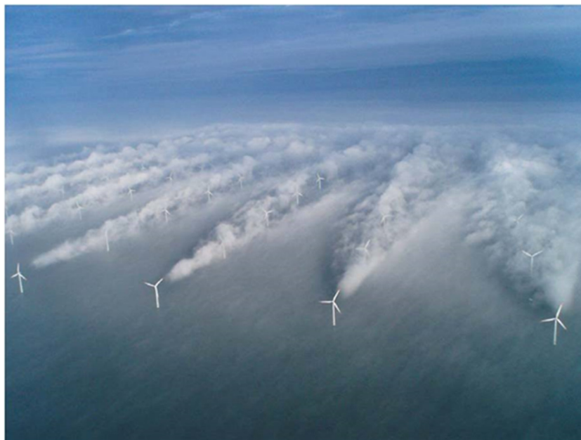
Figure A1. Image taken in February 2018 showing the obvious wake effects marked by humid air condensation in the Horns Rev OWF, Denmark.
