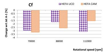
Figure 4. Changes of fuel consumption for synthetic blending components with regard to Jet A-1.
