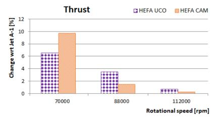
Figure 3. Changes of engine thrust for synthetic blending components with regard to Jet A-1.
