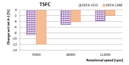
**Figure 5.** Changes of thrust-specific fuel consumptions (TSFC) for synthetic blending components with regard to Jet A-1.
