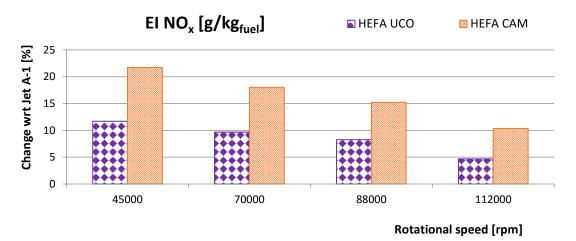
Figure 10. Changes of NO<sub>x</sub> emission index for HEFA blends with regard to Jet A-1.
