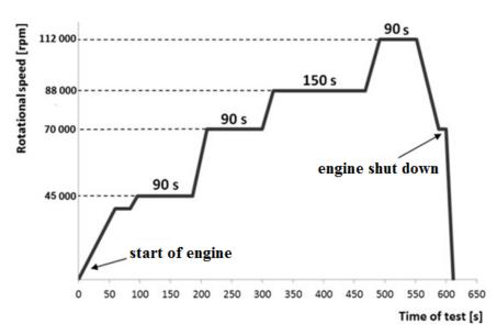
Figure 1. Modified profile of engine test.
