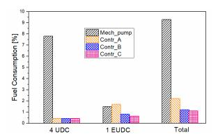
Figure 19. Fuel consumption reduction achieved with the use of the controller during the NEDC cycle.
