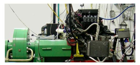
**Figure 4.** Experimental test rig for the 1.2 dm<sup>3</sup> engine.
