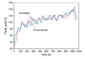
**Figure 7.** The average metal temperature during the New European Driving Cycle (NEDC); comparison between numerical simulations and experimental tests (the temperature at position 11C of Figure 5).
