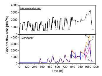
**Figure 15.** Coolant flow rate delivered by the standard belt-driven pump (**top**) and by the various controllers during the NEDC (**bottom**).
