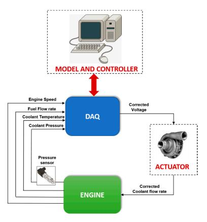
Figure 2. Operating scheme of the controller at the experimental test rig.
