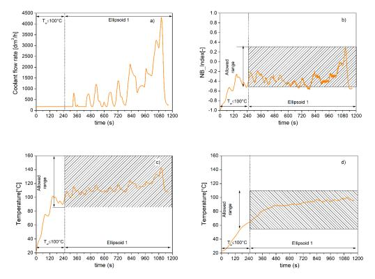
**Figure 10.** Coolant flow rate (**a**), NB\_Index (**b**), wall (**c**), and coolant (**d**) temperature when the controller operates with low boiling levels.
