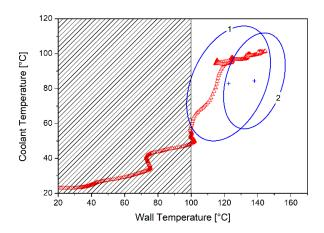
Figure 23 shows that, also for this case, the trajectory falls inside the control regions owing to the fact that the constraints on the input variables, mainly the one on fuel flow rate, are satisfied.
