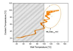
Figure 9. Control region and system trajectory during the NEDC for low boiling levels.
