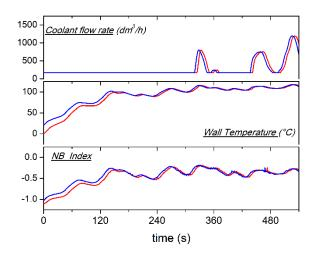
**Figure 21.** Controlled coolant flow rate (**top**), average wall temperature (**middle**) and NB\_Index (**bottom**) during the NEDC cycle starting from 20 °C (red line) and 0 °C (blue line) environment.
