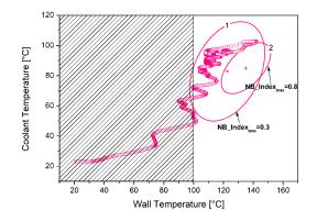
Figure 13. Control region and system trajectory during the NEDC for high boiling levels.
