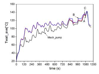
Figure 17. Average metal temperature during the NEDC.
