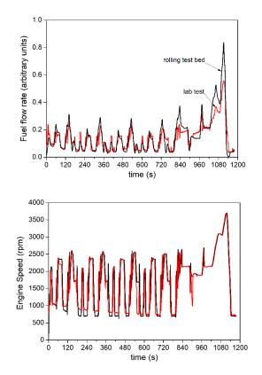
**Figure 6.** Comparison between the rolling test bed and stationary test rig fuel flow rate (**top**) and engine speed (**bottom**) for the 1.2 dm<sup>3</sup> engine.
