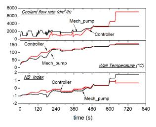
**Figure 26.** Controlled coolant flow rate (**top**), average wall temperature (**middle**), and NB\_Index (**bottom**) for prolonged high load operation ( $\dot{m}_f = 18 \text{ kg/h}$ ).
