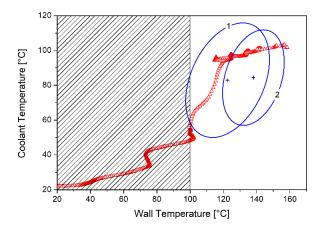
**Figure 25.** Coolant and wall temperatures for prolonged high load operation ( $\dot{m}_f = 18 \text{ kg/h}$ ).
