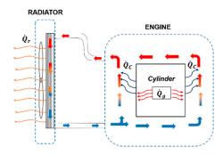
**Figure 1.** Thermal energy fluxes between the in-cylinder gases and the wall  $(Q_g)$  between the walls and the coolant  $(\dot{Q}_C)$  and between the coolant and atmosphere  $(\dot{Q}_r)$  [35].
