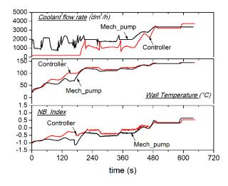
**Figure 24.** Controlled coolant flow rate (**top**), average wall temperature (**middle**), and NB\_Index (**bottom**) for prolonged high load operation ( $\dot{m}_f = 9 \text{ kg/h}$ ).
