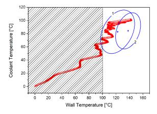
Figure 20. Coolant and wall temperatures during the NEDC starting from 0 °C environment.
