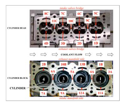
Figure 5. Thermocouple positions in engine head and block.
