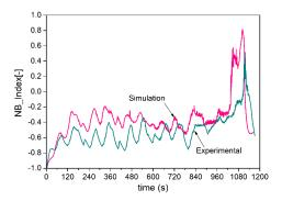
Figure 8. NB\_Index during the NEDC; comparison between numerical simulations and experimental tests.
