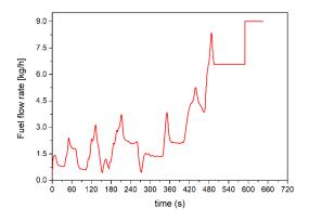
Figure 22. Fuel flow rate variation for prolonged high load operation.
