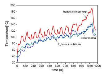
Figure 18. Simulated and measured metal temperatures during the NEDC cycle.
