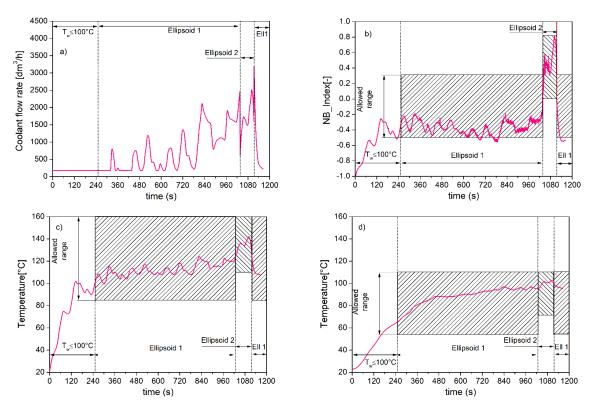
**Figure 14.** Coolant flow rate (**a**), NB\_Index (**b**), and wall (**c**) and coolant (**d**) temperature for high boiling levels.
