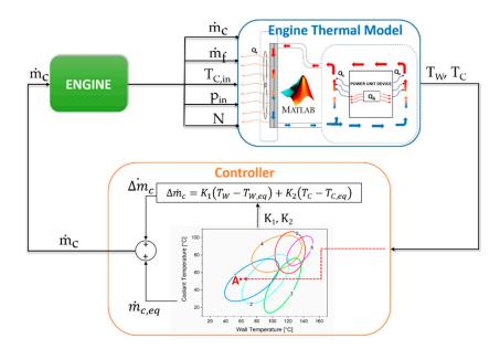
**Figure 3.** Schematic of the interaction between the model and the controller. The variables computed by the model determine the state of the system and define the control stability region.
