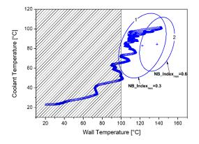
Figure 11. Control region and system trajectory during the NEDC for moderate boiling levels.
