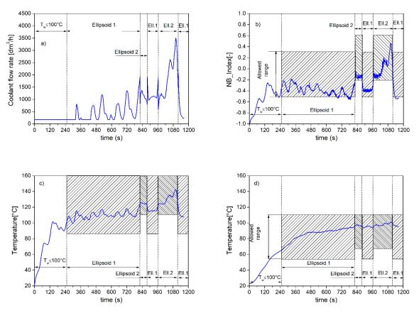
**Figure 12.** Coolant flow rate (**a**), NB\_Index (**b**), and wall (**c**) and coolant (**d**) temperatures for moderate boiling levels.
