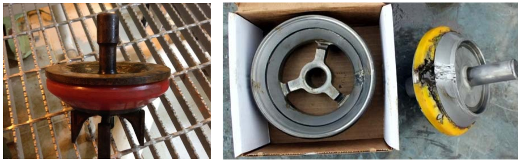
Figure 7. A new valve head (left) and damaged seat and head of a mud pump valve (right) [4,6].
