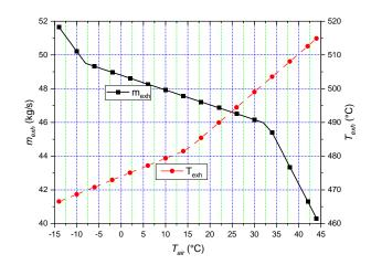
Figure 3. Mass flow rate and temperature exhaust from GE10 gas turbine, varying ambient temperature.
