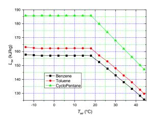
Figure 11. Expander specific work varying ambient temperature.
