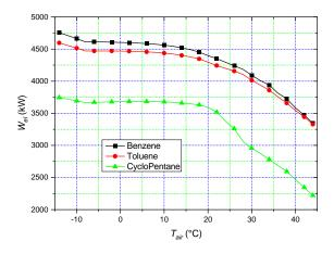
Figure 4. ORC electrical output power varying ambient temperature.
