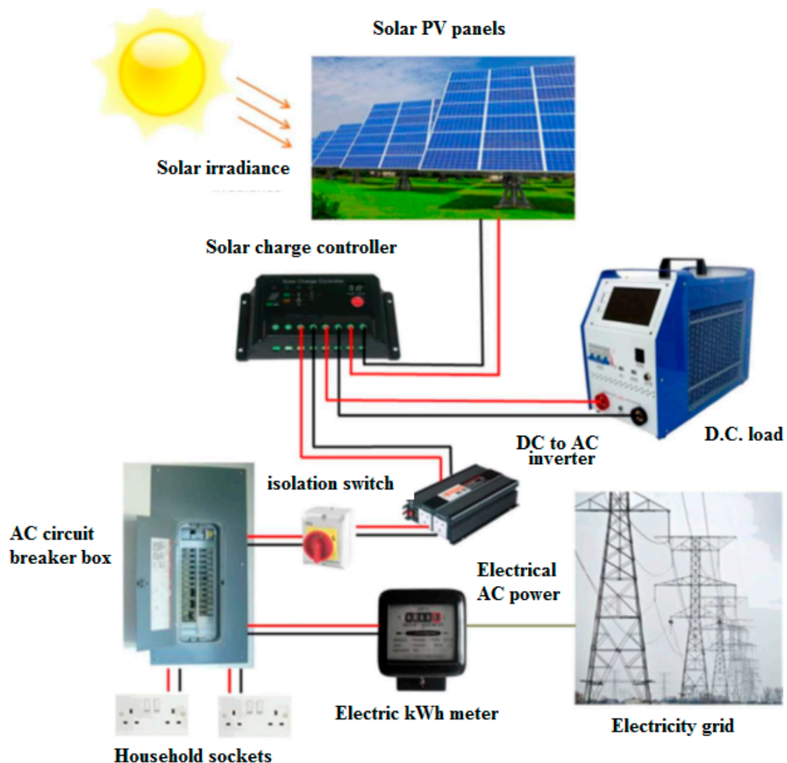
Figure 5. Components of the grid-connected photovoltaic (PV) system.
