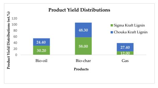
**Figure 3.** Product yield distributions (wt.%) of fast pyrolysis of Sigma Kraft (softwood) and Chouka Kraft (hardwood) lignin.
