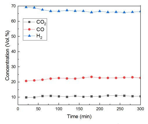
**Figure 4.** Gas product concentration at 800 °C, S/C:3, GHSV:61,200 h<sup>-1</sup> in a 5-h test.
