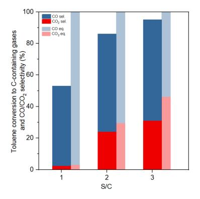
**Figure 6.** Toluene conversion to C-containing gases and CO/CO<sub>2</sub> selectivity at different S/C ratios (GHSV:61,200  $h^{-1}$ , 800 °C).
