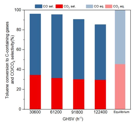
**Figure 5.** Toluene conversion to C-containing gases and CO/CO<sub>2</sub> selectivity at different GHSVs (S/C:3, 800 °C).
