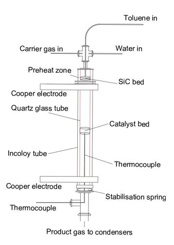
Figure 2. Reactor diagram of catalytic toluene steam reforming.
