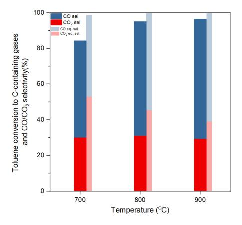
**Figure 3.** Toluene conversion to C-containing gases and CO/CO<sub>2</sub> selectivity at different temperatures (S/C:3, gas hourly space velocity (GHSV):61,200  $h^{-1}$ ).
