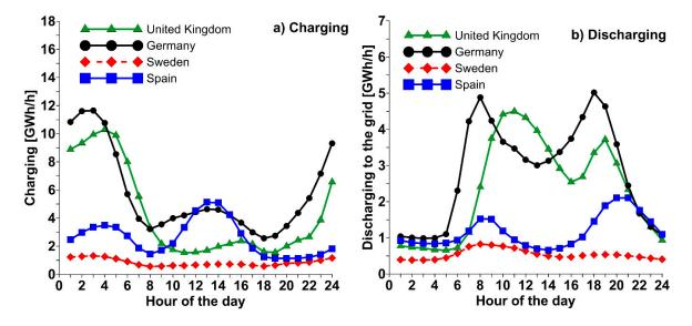
**Figure 7.** Levels of charging (**a**) and discharging back to the electricity grid (**b**) for the EV fleet for an average day in the four investigated countries.
