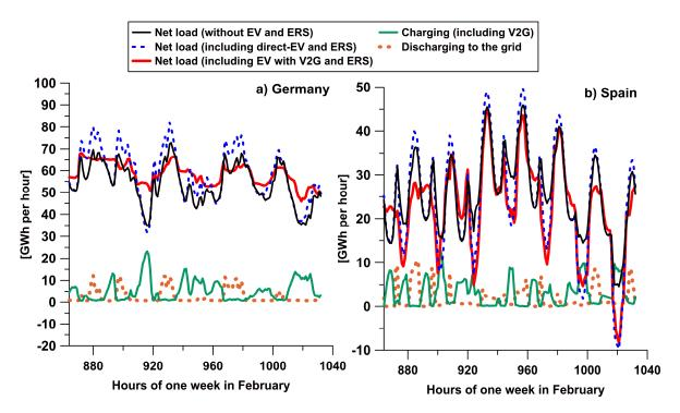
**Figure 6.** The net load without EVs and ERS (i.e., the load minus useful solar and wind electricity generation), the net load including direct charging of EVs and ERS for trucks and buses, the net load including EVs with V2G and ERS, and the load from charging and discharging to the grid are shown for 1 week in February for (**a**) Germany and (**b**) Spain.
