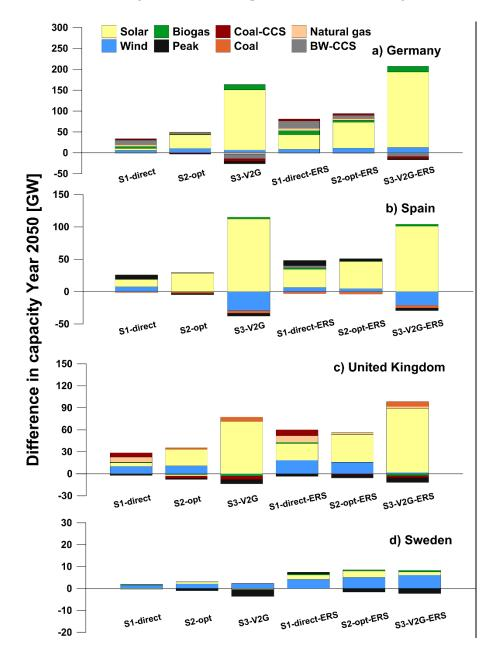
**Figure 4.** The differences in installed capacity Year 2050 between a scenario without EVs and the various EV and ERS scenarios investigated for: (a) Germany; (b) Spain; (c) the UK; and (d) Sweden. Opt, Optimisation of EV charging; CCS, carbon capture and storage; V2G, vehicle-to-grid; ERS, electric road system; BW, lignite co-fired with biomass.
