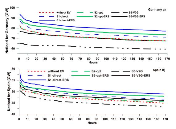
**Figure 5.** The net-load curves in Year 2030 sorted with respect to the 168 h with the highest net loads in: (a) Germany; and (b) Spain.
