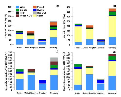
**Figure 3.** Installed capacity Year 2050 for the four countries investigated in the scenarios (**a**) without electric vehicles and (**b**) S3-V2G; and electricity generation Year 2050 for the four countries investigated in the scenarios (**c**) without electric vehicles and (**b**) S3-V2G. CCS, carbon capture and storage; BW, coal co-fired with biomass.
