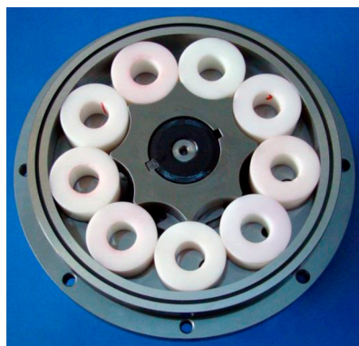
Figure 26. The conventional outer rotor replaced by rollers (Heisel and Mishev [164]).
