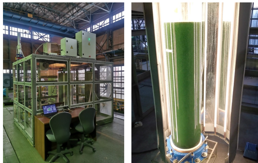
Figure 2. A view of atmospheric gas chamber (AGC) with a photobioreactor (PBR) inside the chamber.
