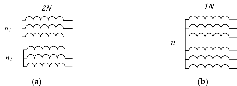
Figure 4. (a) Two neutral connections; (b) A single neutral connection for six-phase machine winding.
