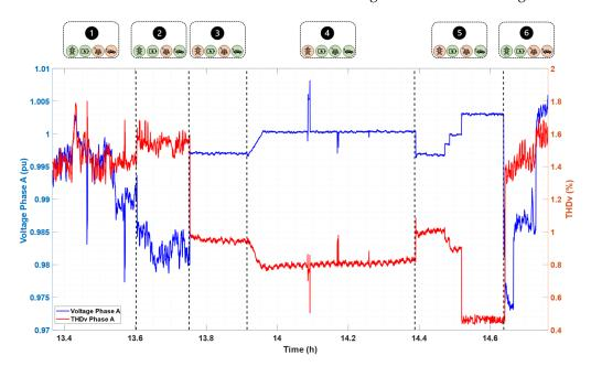
Figure 7. Voltage and voltage harmonic distortion of the system collected by power analyzer.
