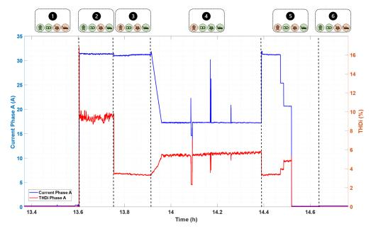
Figure 8. Current and current harmonic distortion of the system collected by power analyzer.
