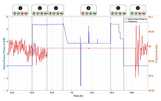
Figure 6. Active power and system frequency collected by power analyzer.
