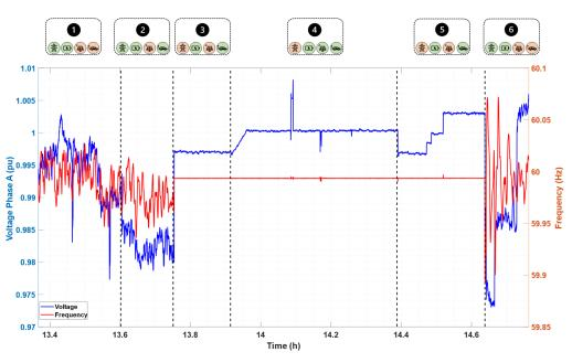
Figure 5. System voltage and frequency collected by power analyzer.
