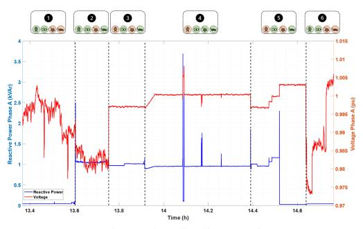
Figure 9. Reactive power and system voltage collected by power analyzer.
