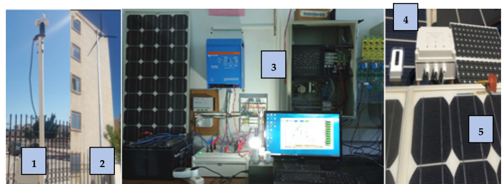
Figure 6. Measurement acquisition device at the laboratory. Where: 1: wind speed sensor, 2: wind turbine, 3: data acquisition system, 4: solar irradiance and ambient temperature sensor, and 5: PV panel.
