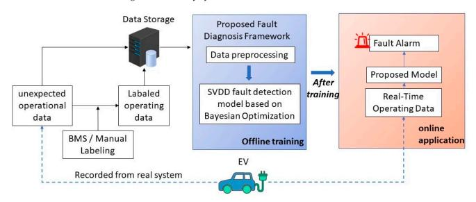
Figure 16. Fault detection proposed application for EV battery by [155].
