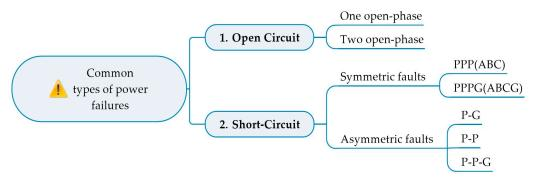
Figure 3. Common types of power failures (open circuit and short circuit failures).
