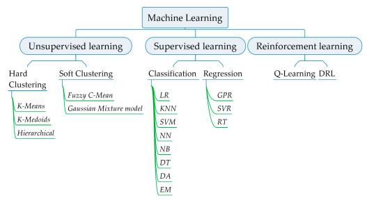
Figure 9. ML techniques for fault diagnosis in EPS [95].
