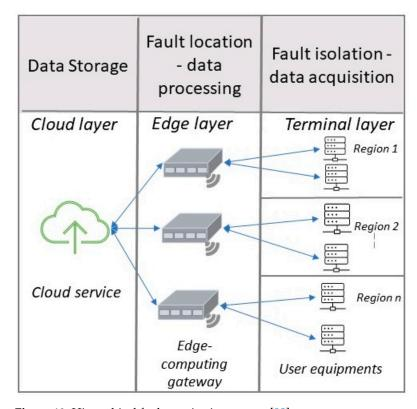
Figure 10. Hierarchical fault monitoring system [98].
