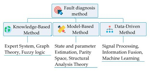
Figure 15. Fault diagnostic methods classification [149].
