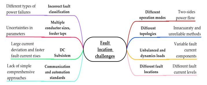
Figure 2. Fault location challenges in SG's distribution domain [21].
