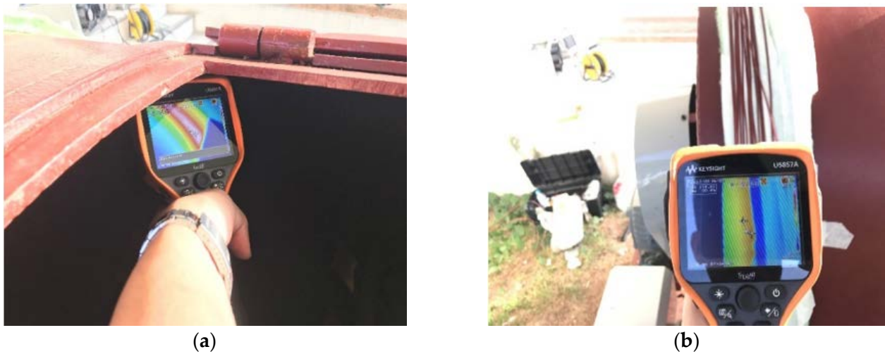
Figure 9. (a) The temperature inside the tank in the copper wire area. (b) The temperature outside the tank around the copper coil area.
