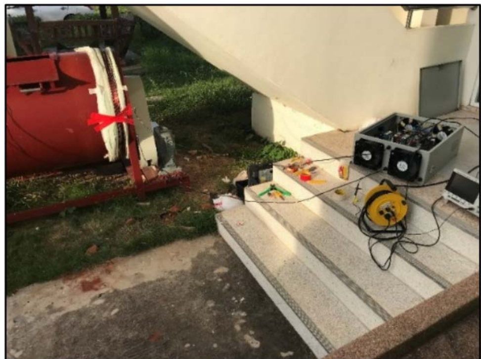
Figure 8. Heat induction machine applied to large bioreactor.
