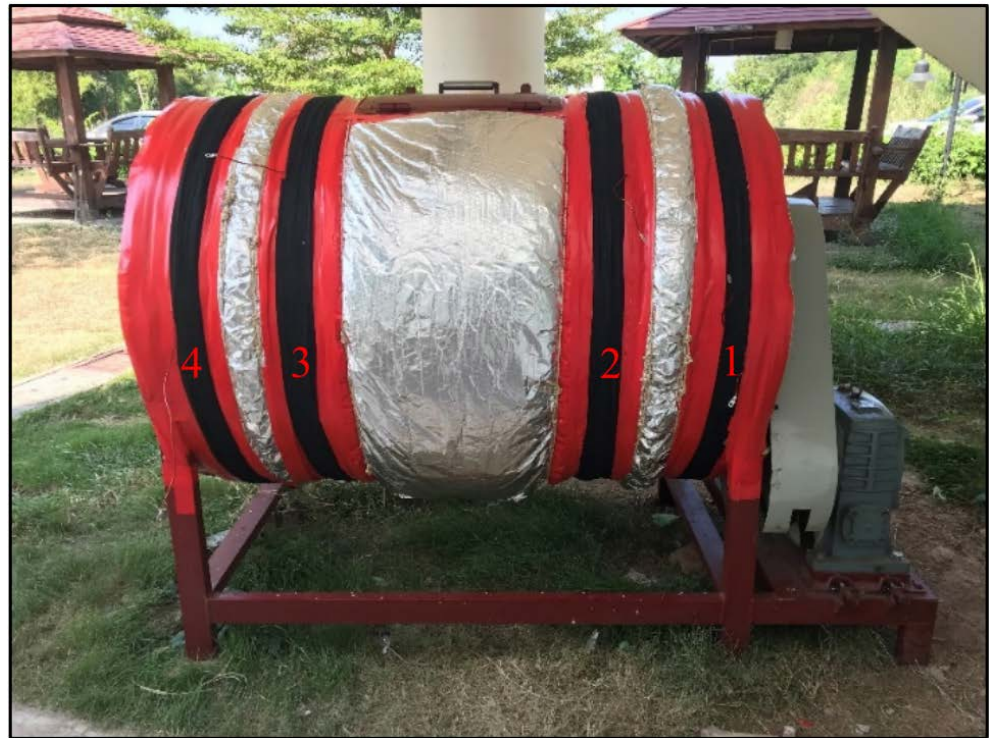
Figure 11. Four sets of wire-wrapped heating bins ready to be used for heating and decomposing organic waste.
