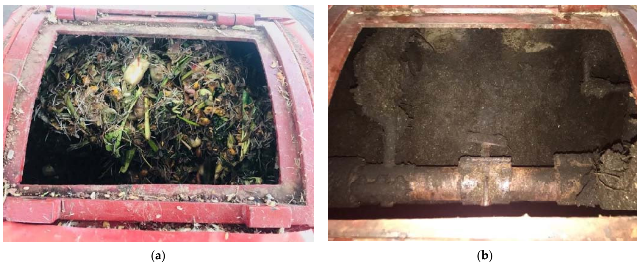
Figure 17. (a) The total of the waste weighted into the bioreactor. (b) After 20 h of heating, the temperature of the material was 90 °C.
