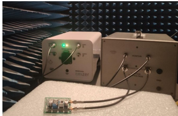
Figure 13. CE measurement setup, which contains a EUT (front row), an EMSCOPE (a two-port EMI receiver, background, left side), and a two-port LISN (background, right side).
