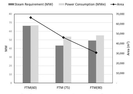
**Figure 4.** Effect of steam temperature on membrane area, steam flow rate and energy requirement at fixed 90% recovery and 95% purity of the captured CO<sub>2</sub>.
