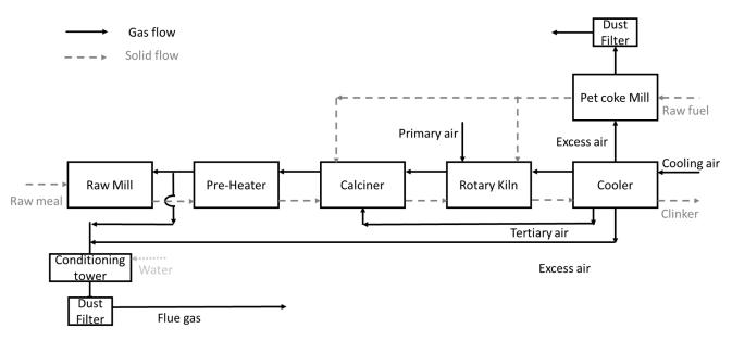
Figure A1. BFD (Block Flow Diagram) of the real clinker production plant in Gubbio, Italy.
