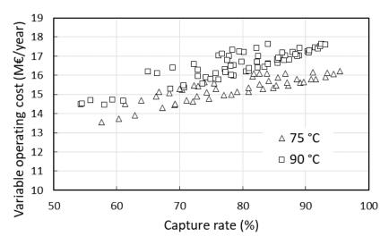
Figure 7. Effect of capture rate on the variable operating costs of the plant at different steam grades.
