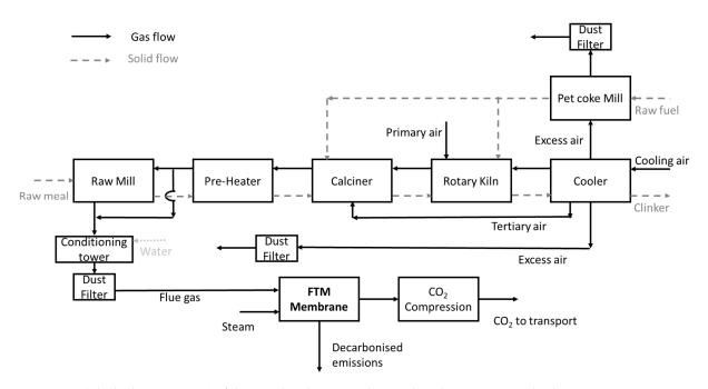
**Figure 1.** BFD (Block Flow Diagram) of the simulated cement plant with carbon capture and subsequent  $CO_2$  compression. The BFD for the production section is modified compared to the real plant as the excess gas from the cooler is not mixed with the gas stream form preheaters and raw mill; the carbon capture and compression sections are added in the simulation to this gas stream.
