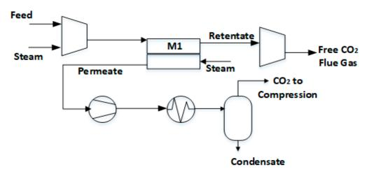
Figure 2. Simplified PFD of FTM technology for carbon capture considered in the simulation.
