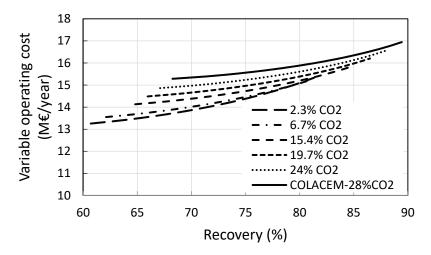
**Figure 8.** Effect of CO<sub>2</sub> molar fraction at the inlet of the membrane module on the variable operating costs at fixed sweep flow rate.
