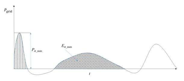
Figure 7. Qualitative visualization of energy storage systems sizing approach.
