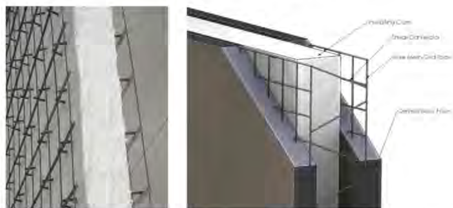
Figure 3. Details of a typical cementitious sandwich panel with individual welded wire shear connectors ( Class I ).
