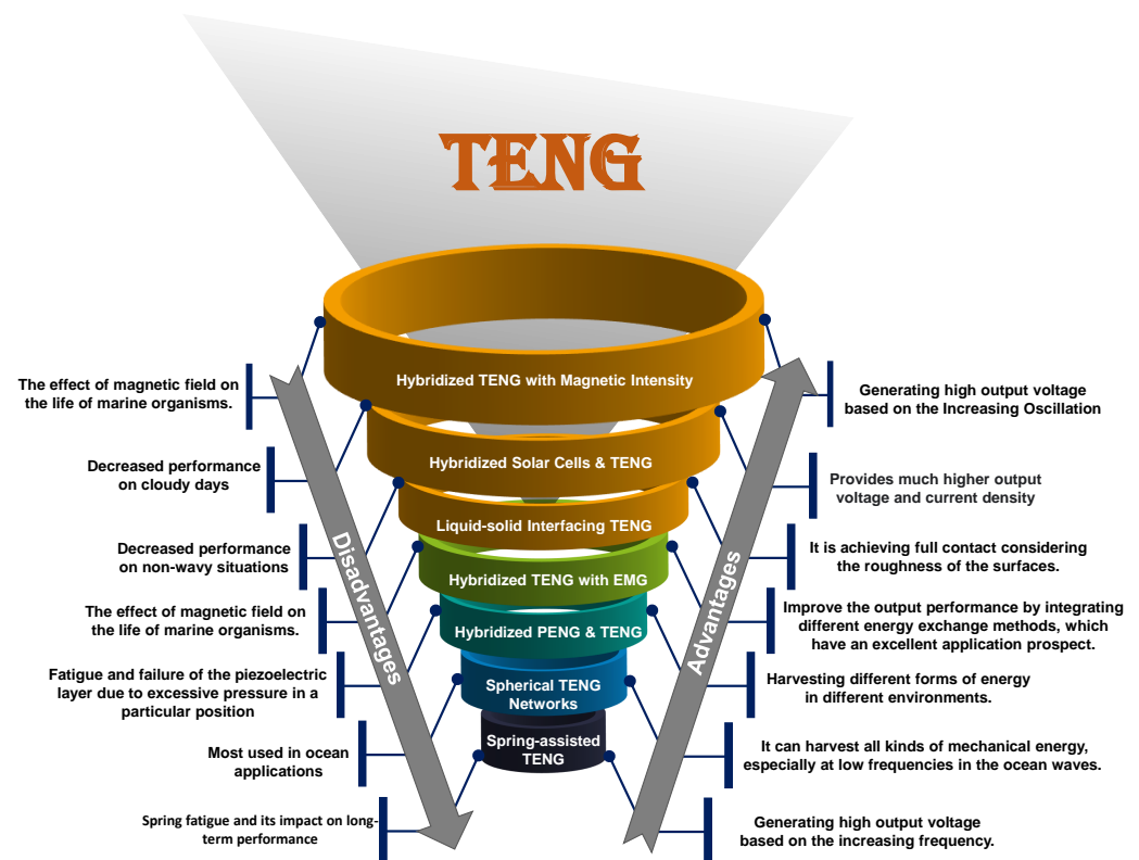
Figure 13. Advantages and disadvantages of different TENG structures.
