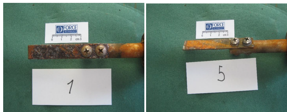
(a) Steel coupon exposed for 5 months
