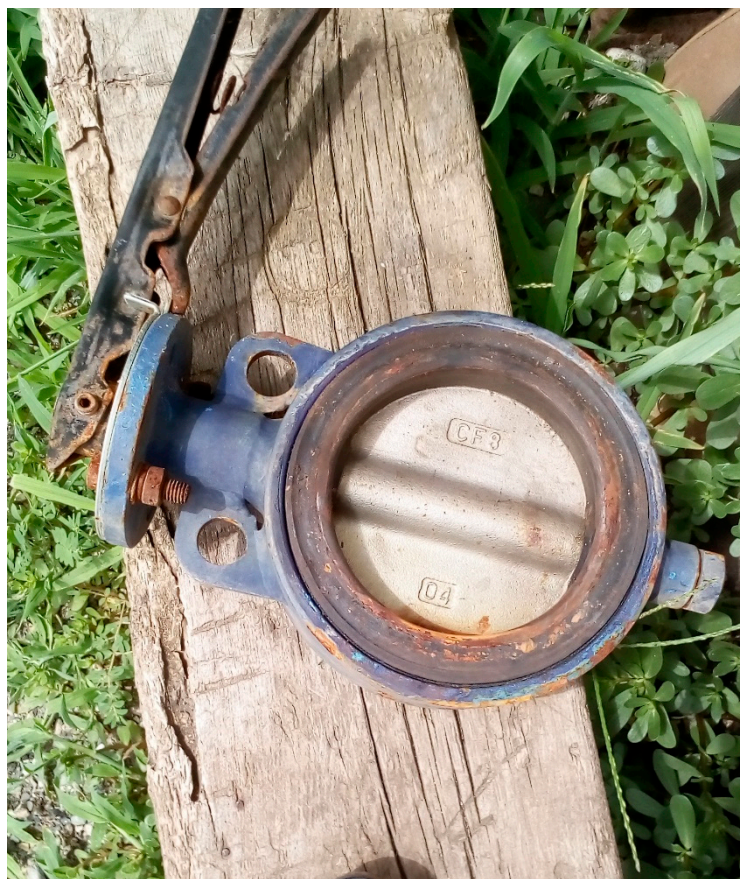
Figure 21. The appearance of the valve installed in the geothermal heating system with an acoustic–magnetic device.
