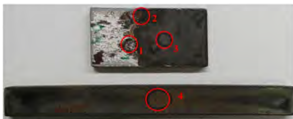
Figure 11. Macrostructure of the corroded sample at 65 °C.
