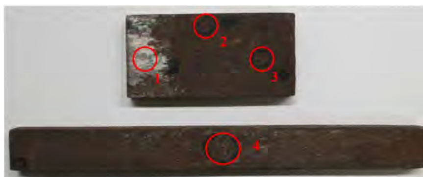
Figure 4. The samples prior to SEM/EDS analysis with indicated analysis points.
