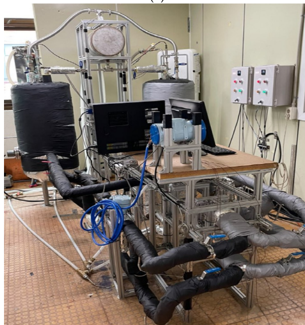
Figure 1. Schematic diagram and the image of experimental setup. (a) Schematic diagram of experimental setup: (1) Solution tank, (2) Condenser, (3) Test PHE, (4) Recovery PHE, (5) Cooling PHE, (6) Constant temperature bath, (7) Solution pump, and (8) Mass flow meter. (b) Image of experimental setup.
