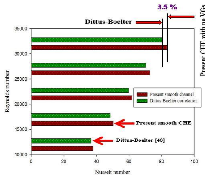
Figure 3. Nu values for an unbaffled duct.
