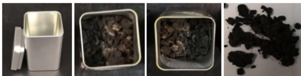
Figure 1. The sewage sludge and biochar samples example. From the left, the crucible, raw SS sample in the crucible, biochar from SS in the crucible, and produced biochar from SS.
