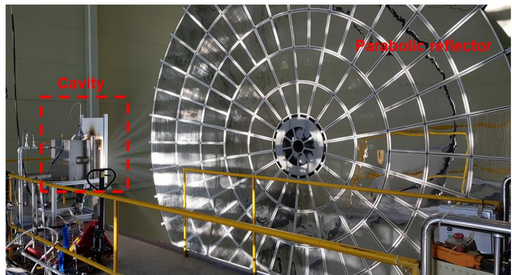
Figure 5. Installed reactor in a solar furnace.
