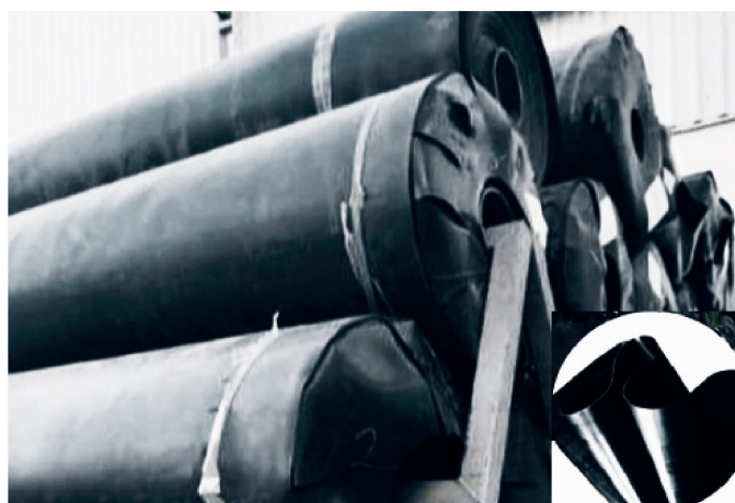
Figure 1. Geomembrane used in the manufacture of biodigesters.
